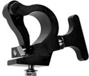
The new standard truss clamp for hanging intelligent lighting fixtures. Allows one man to hang intelligent fixtures. Simply flip the link up, place the clamp over the pipe and the Mega-Claw holds the weight of the fixture while you secure it with the solid 3/4" thick handle. The Mega-Claw will fit onto (1-1/2" Pipe) 1.9" OD to 2" OD.
