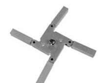
The Mega-Folding Floor Stand is a compact folding stand for placing light fixtures on the stage floor. It folds out into a stable 15" light base and folds up into a 6" square. Just fold in the appropriate legs to fit into corners, tight spots and against walls. The Mega-Folding Floor Stand has replaceable rubber feet so it won't mar the stage floor. A 1/2"-13 tpi x 1" long hex head bolt fastens the light fixture to the Mega-Folding Floor Stand. Available in either mill or black finish.
