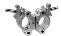
The Swivel Coupler will fasten from 1-1/4" pipe (1.660" OD) to 2.050" OD truss tube. The Swivel-Coupler has wide wing nuts for fastening the clamp to the pipe or tube.
