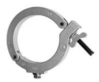
The Monstro-Couplers are designed to fit pipes larger than the standard theatrical battens. CNC machined from solid billet aircraft-grade aluminum, they are perfect for attaching to odd size pipes and tubes. Monstro-Couplers have a narrow size range of application. They are designed with a plus or minus 0.0625" tolerance on their nominal size to ensure that they will fit with the Aluminum Association pipe and tubing manufacturing tolerances. Custom sizes are available upon request.
