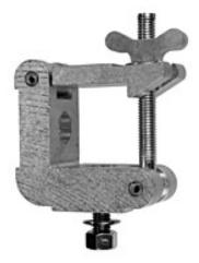
Fits 2" Square Tubing. Notched to bolt onto 2" square tubing. Fastens with standard ½" bolts 6061-T6 Aluminum,
