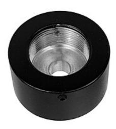
The 5/8" Bolted Truss to Pipe Adapter easily allows joining a pipe to the end of a 5/8" bolted truss. Simply bolt the adapter to the truss with a 5/8" bolt and thread on a 1-1/2" pipe for special requirements. Locking set screw for pipe threads for extra safety.
