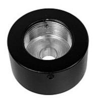
The 5/8" Bolted Truss to Pipe Adapter easily allows joining a pipe to the end a 5/8" bolted truss. Simply bolt the adapter to the truss with a 5/8" bolt and thread on a 1-1/2" pipe for special requirements. Locking set screw for pipe threads for extra safety.
