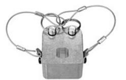
The Chandelier Chain Mount is CNC machined from 6061T-6 aluminum and attaches with two stainless steel 3/8" x 1.5" ball detent pins through the Chandelier Chain Mount and the hollow chain link pins to secure  $\frac{1}{2}$ " square bar or tube chandelier mounts anywhere along the length of the chain.
