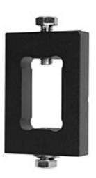
The Genie Fork Adapter is supplied with a 1/2" x 1" Grade 5 bolt and Belleville spring washer to fasten the load to the adapter. An additional 1/2" bolt locks the adapter to the Genie fork. The adapter also fits a Sumner Fork. The Genie Fork Adapter is sold individually (not in pairs).
