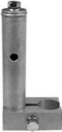
Light Mount Kit for 2" Pipe Fence Post fits 2" pipe fence posts, provides a 3/4" bolt to mount outdoor light fixtures, and also provides a 1/2" conduit threaded connection in the 2-3/8" OD by 12" long tube for wiring the light fixture.
