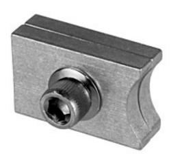
M140 Track Stop for M140 Track. Two CNC machined 1/4" x 1" aluminum flat bars with contours that match the curviture of the M140 Curtain Carrier, so as not to "ding" the carrier wheel. The rear bar is threaded for a 5/16" socket head screw to fasten the track stop to the track without needing a nut. The M140 Track Punch will quickly and efficiently add a hole to mount the M140 Track Stop.
