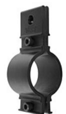
The two-piece, Mega Batten Clamp is great way to hang 1-1/2" pipe. The tight compression fit keeps pipe from rotating within the clamp. The Mega Batten Clamp wraps around the pipe batten on both sides and fastens with two 5/16"-18 TPI socket cap screws using a 1/4" hex driver. Secure to structural supports through nominal 1/2" hole at top of clamp with up to a 7/16" shackle pin, quick link, or turnbuckle jaw. CNC Machined 3/16" thick x 2" wide 6061T-6 Aluminum.
