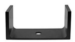
The Mega-Cable Carrier gives you a channel to drop your cables into above the batten or grid. The Mega Cable Carrier has a 1/2" mounting hole and is bolted to a clamp. The assembly is then fastened above a pipe batten or grid to run cables. The cables are then located over the pipe, giving you clearance to hang your lights without having to fight the cables, or to worry about messy tie lines.
