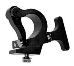
The new standard truss clamp for hanging intelligent lighting fixtures. Allows one man to hang intelligent fixtures. Simply flip the link up, place the clamp over the pipe and the Mega-Claw holds the weight of the fixture while you secure it with the solid 3/4" thick handle. The Mega-Claw will fit onto (1-1/2" Pipe) 1.9" OD to 2" OD.
