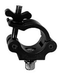
The Mega-Coupler has solid wing nut tabs that are stronger than regular steel wing nuts. The grade 8 Hex Head Cap Screw locks securely into the hex milled pocket so that the Nylock Nut can be tightened while the clamp is installed
