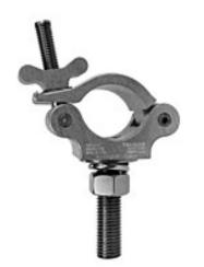
The Mega-Coupler with a 3/4" -10 tpi x 3/12" steel stud is great for hanging large commercial lighting fixtures to 1-1/2" pipe.
