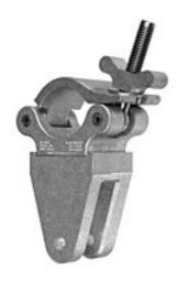
The Mega-Coupler with Clevis attachment is CNC machined from 6061T-6 aluminum. 3/8" cross bolt hole for attachments. Will bolt to the Mega-Coupler either parallel with the pipe or perpendicular to the pipe.
