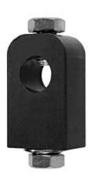
The Mega-Drop Down Slider works with The Light Source Mega-Drop Downs to locate light fixtures along the length of the Mega-Drop Down. Two 1/2"-13 x 1" long Hex Head Cap Bolts both mount the fixture and lock the fixture onto the Mega-Drop Down. A nickel plated, spring steel 1 inch OD Belleville spring washer is provided to act as both a tensioning and locking washer. CNC machined from aircraft grade aluminum
