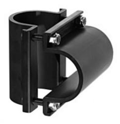
The Mega-Gridlock is designed for permanent installations in studios and theaters. It joins 2 overlapping pipes together in a 90 degree joint. The side grooves act as a wrench, keeping the nut from turning during installation.
