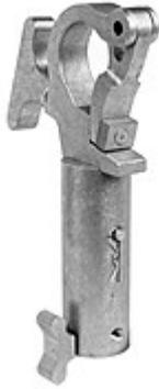
The Mega-Junior Pin Receiver is a great way to hang your film and studio light fixtures! Fits the standard 1-1/8" spuds commonly used for light stands and allows you to utilize these fixtures on the studio grid pipes. The Slim-Claw fits 1-1/2" pipe (1.9" OD) and 2" tubing without needing hand tools to hang the light fixture to the grid.
