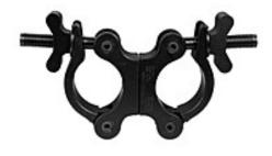
The Mega-Slim Swivel Coupler is a light weight option for less demanding rigging needs. It is half the thickness (1") of our standard Mega-Coupler and weighs 30% less; yet fits the same range of diameters as the Mega-Coupler.
