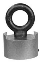
The Mega-Tie Off is used backstage for securing boom base pipes to the grid for safety. The 1/2" eye bolt swivels 360 degrees. The Mega-Tie Off has 1.5 NPT pipe threads and a 1/2" two-way lock nut secured with permanent Loctite.
