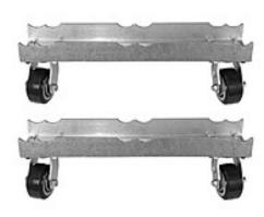
The Mega-Truss Dolly easily holds truss for transport or storage. The 5" aluminum C channel has CNC milled cutouts for truss to ride in. It is important to secure the trusses tightly to the Mega-Truss Dolly with an E-Clip ratchet strap before moving.
