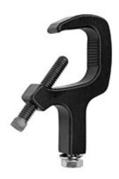
The Micro Clamp is ideal for hanging miniature fixtures like MR-16's onto a small pipe or tube. Made from high tensile aircraft aluminum. Solid design grips pipe with micro grooves, has spring loaded pan adjustment, and has 5/16" fasteners. Available in black anodized, or polished aluminum finishes.
