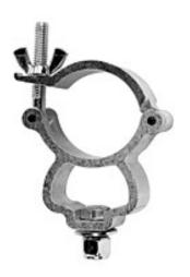
The Mini-Coupler is 1" wide and fits from 1.65" OD to 2" OD Tube. The Mini-Coupler uses a 3/8" x 3/4" long Grade 5 bolt with a Belleville washer and a Nyloc nut. The Mini-Coupler has a safe working load of 330 Pounds. (150 Kg)
