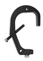
The Monstro-Clamp 4" fastens to 2-3/8" OD to 4" OD pipes. CNC cut from solid one inch thick aluminum plate. 1/2"-13 x 4" square head bolt.
