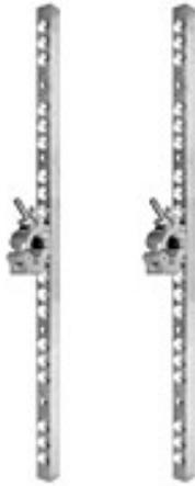
The Plasma Universal Mount supports a plasma or LCD screen on a pipe, 12", or 20.5" Truss. One Quad-Coupler 1.5 is provided to fasten per mount. The two mounting bars are bolted directly to the plasma screen with two 8mm or 10mm bolts per bar. The support bolt holes are drilled for the 50, 100, 150, 200, 300, 400, 600 mm VESA Standards. Priced per set.
