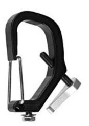
Perfect for high catwalks and educational facilities with less experienced crews. Snaps onto the pipe with a carabineer style latch and cannot fall off. (except off the end of the pipe!) Easily fastens to 1-1/4" Pipe (1.66" OD), 1-1/2" Pipe (1.9" OD), and 2" truss tube with included handle.
