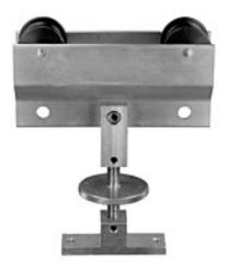
The Scenery Carrier is adjustable to fine tune the height or leveling of your flats or other scenery elements. Turnbuckle style bolt makes for quick adjustments by turning the knurled disk. Two holes are provided for #10 wood screws.
