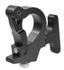
The Slim-Claw will fasten to both 1-1/2" pipe (1.90" OD) and 2" OD truss tube. The Slim Claw has a 3-1/2" T-handle, so no tools are required to fasten to the pipe. Comes with 1" x 1/2"-13 TPI Grade 5 fastener and 1" diameter Belleville Spring washer.
