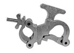
The Slim Claw to Mega-Coupler 1/2 CS makes an easy job of hanging a lamp bar to truss. Pre-fasten the Mega-Couplers to the lamp bar. When on site for the event, simply hook the Slim-Claws onto the truss/pipe and fasten the link and handles. The Slim-Claw supports the load while the link is being secured.
