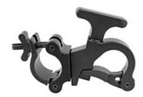
The Slim Claw to Mega-Coupler 1/2 CS makes an easy job of hanging a lamp bar to truss. Pre-fasten the Mega-Couplers to the lamp bar. When on site for the event, simply hook the Slim-Claws onto the truss/pipe and fasten the link and handles. The Slim-Claw supports the load while the link is being secured.
