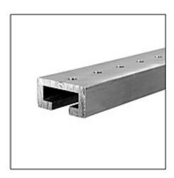
The XYZ Channel and the XYZ Mount make installing LED video walls a breeze. The 6061T6 aluminum alloy channel is pre-drilled on one inch centers for number 12 flathead screws to allow easy mounting to 16" and 24" on center studs. The XYZ mount slides in from the side to any desired location and is locked in place with a set screw. Available in two lengths, 1800 mm and 2400 mm, to match most LED panels.
